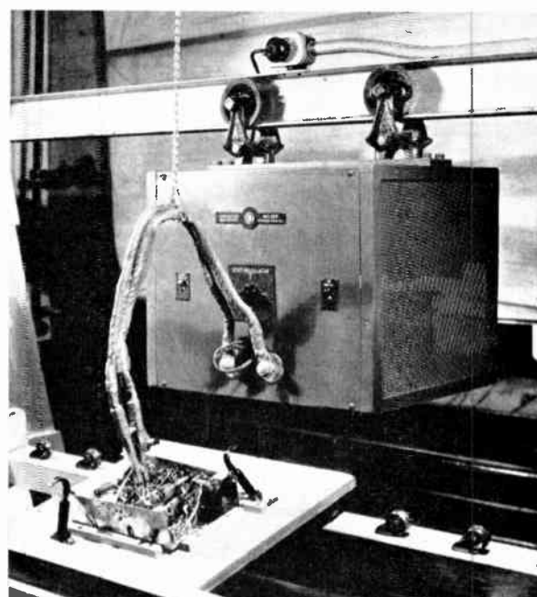
Fig. 131. Capacitor welder on radio receiver production line, for welding of connections
