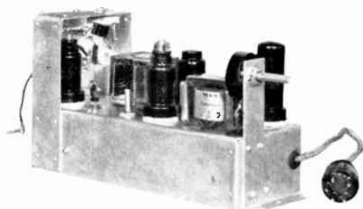
Fig. 129. Ultra-high-frequency receiver for police motorcycles
