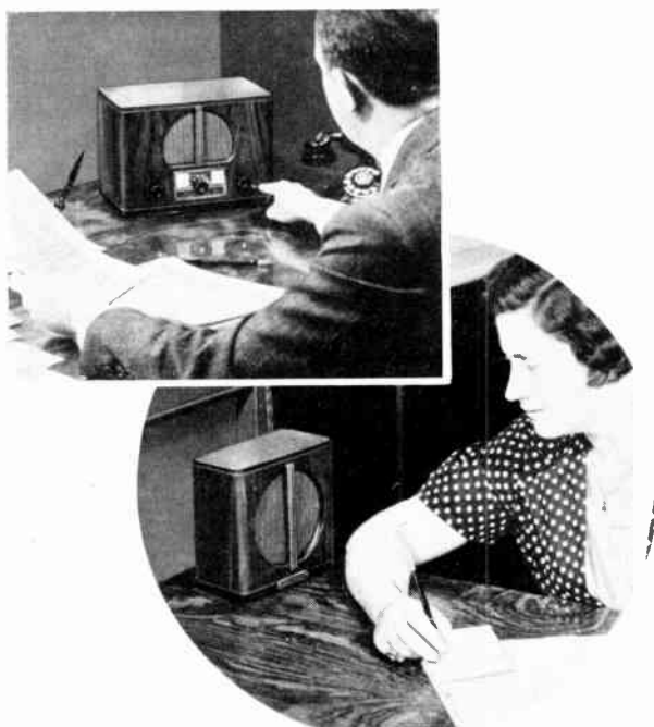
Fig. 127. Intercommunication system: (upper) master station; (lower) remote speaker-phone station
